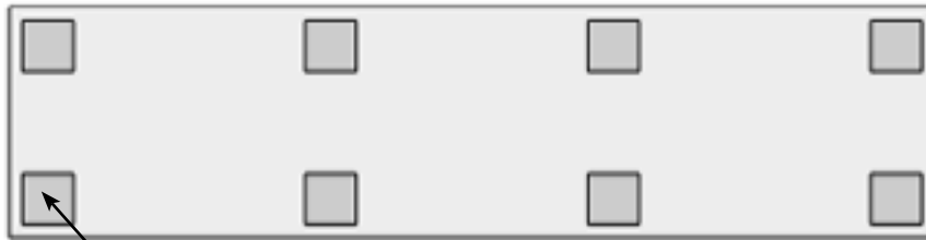
(8) Pads, 4"x4"x1/8"thk. Offset 1" from edges.
