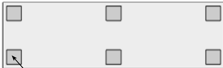
(6) Pads, 4"x4"x1/8"thk. Offset 1" from edges.
